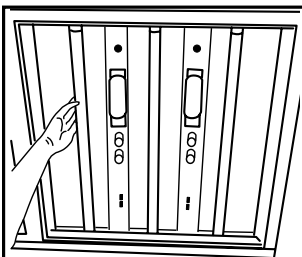
1 Remove the fluorescent Tubes & ballast
